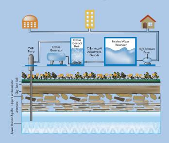
Well pumps at OUC's water treatment plants draw water from a natural underground reservoir called the Lower Floridan Aquifer. After being sent through ozone treatment basins, the water is treated with chlorine and fluoride. The water is then pumped to a finished water reservoir, where it waits for distribution to residential, commercial and industrial customers. Each year OUC delivers nearly 30 billion gallons of water to customers across a 200-square-mile territory.
